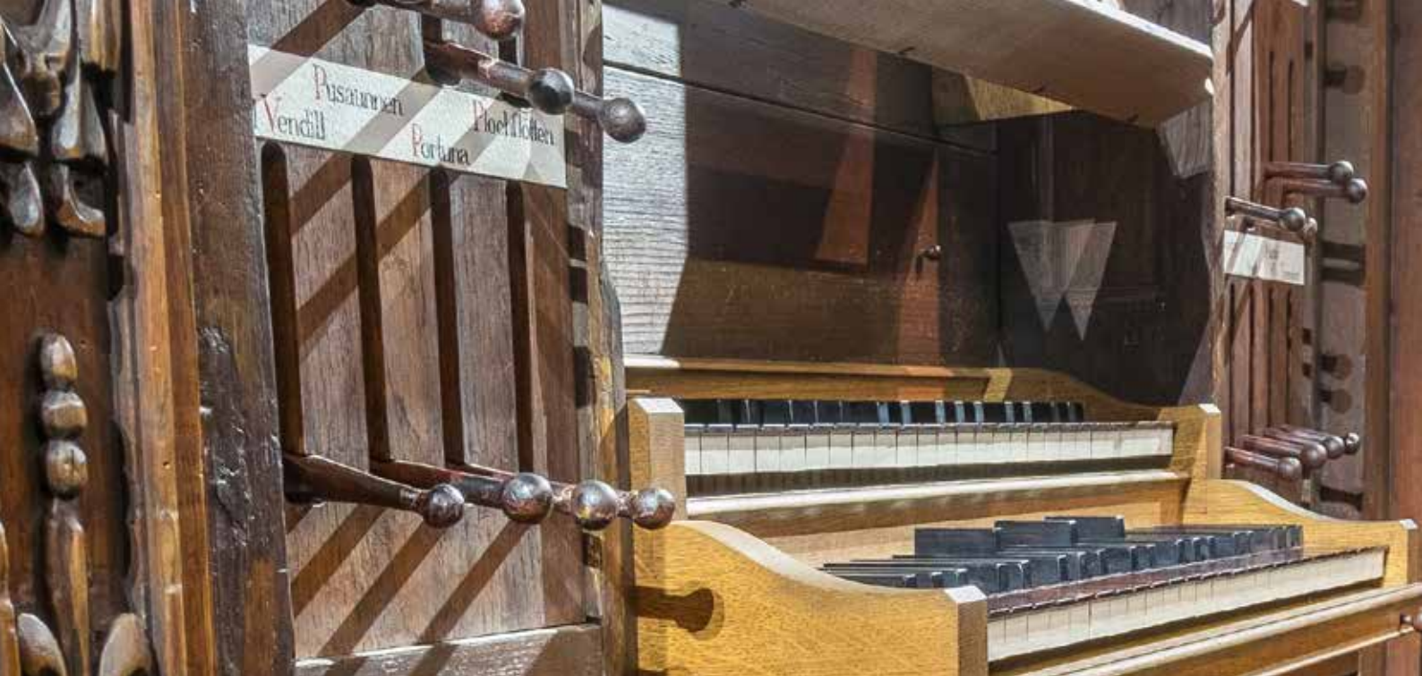
The Wöckherl organ (1642) of the Franziskanerkirche Vienna (with split sharps for g\#^0/ab^0 , d\#^1/eb^1 und g\#^1/ab^1 ) | photo: Norbert Kindermann
